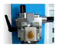
Sample orientation is simple and precise; when the red spot is visible, the orientation plane is at zero. The steel quick-clamp is equipped with a device for quick change of cassettes without altering the inclination of the sample.
