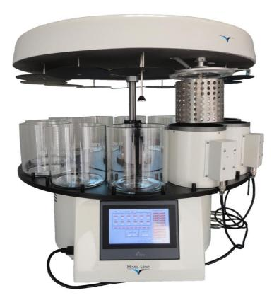
Constant temperature controlling system adopted on the paraffin tank to ensure high precision of temperature controlling, nonstick TEFLON coating painted on the internal surface that provide the good condition for tissue protection. The individual covers for each one of the vessel reduce the emission of vapors to a minimum.
