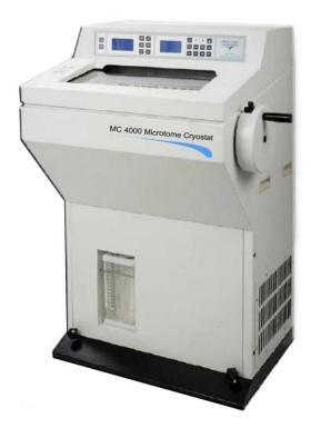
This unique dual compressor semiautomatic cryostat, is equipped with double cooling circuit that allows user to set temperature of specimen differently from cryochamber and shelter temperature.
