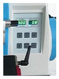
The automatic feed of the sample is controlled precisely by the side electronic panel. The hand wheel allows to set the automatic speed of execution of cutting through a speed variator from 0 to 55 rpm, to allow an excellent and more precisely automatic section results even for difficult tissues. The sample retraction can be set in value by user.
